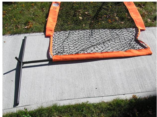
2. The bottom edge of the net forms a fabric sleeve. This sleeve is slid over the straight metal tube.
