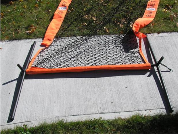
3. The second leg tube is snapped onto the other end of the straight tube.
