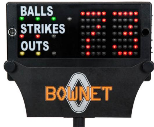
16. Batteries must first be installed in the electronic module as described below. The electronic display module is attached to the plastic holder on top the tripod using two thumb screws. The screws should be firmly hand tightened; tools are not required.
